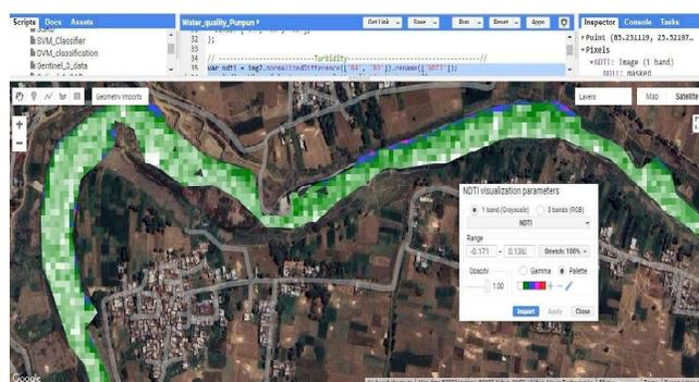
Fig.2. Run the classification algorithms in google earth engine.
