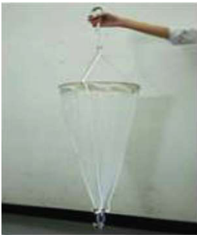
Fig. 1- Plankton net (mesh size: 20 \mu\text{m} for phytoplankton and 60 \mu\text{m} for zooplankton)
