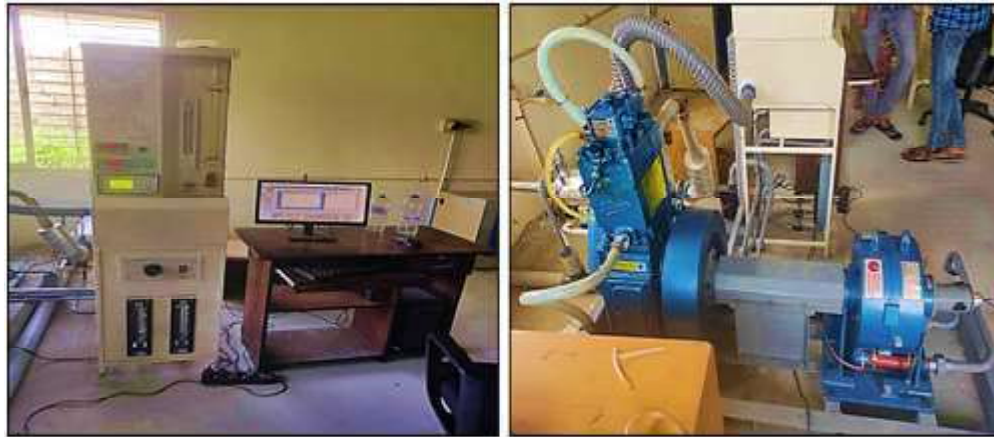
Fig. 3.2: Computerized Single Cylinder 4 Stroke Diesel Engine
