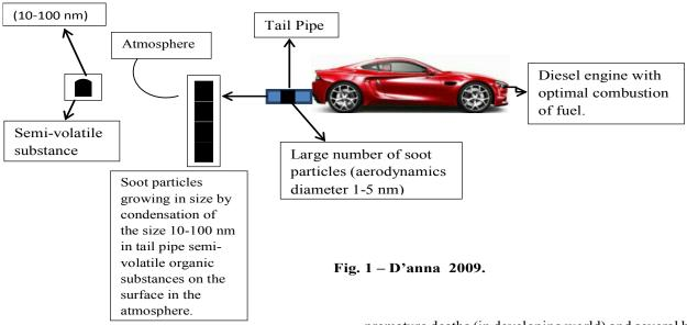
A) When fuel undergoes optimal combustion at high temperature (as in diesel engine), emits large number of small soot particles (aerodynamic diameter being 1-5 nm). These soot particles grow in size (10-100 nm) in tail pipe and undergoes simultaneous condensation of semi-volatile organic substances in the atmosphere.<sup>3</sup> (Fig. 1) He further opines that the speed of growth is dependent upon air temperature, sunlight & the concomitant oxidants etc.
