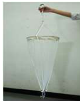
Fig 1 :-Phytoplankton net (mesh size:50-80 \mu\text{m} )
