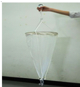
Fig 1 :-Phytoplankton net(mesh size:20-40 \mu m)
